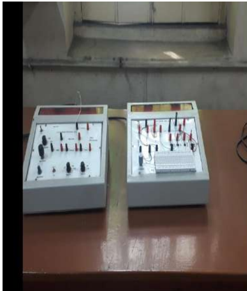
KIT FOR THE MEASUREMENT OF PLANCK'S CONSTANT
